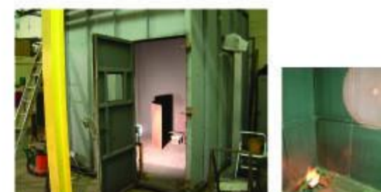
IEC 61034 Smoke Density Test
