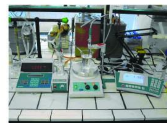
IEC 60754-2 Gas Acidity Test
